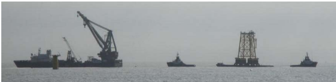
Seaway Heavy lifting's STANISLAV YUDIN with on the right the PEGASUS and BREMEN FIGHTER with the DOW jacket as seen from the AHT UNION PRINCESS – Photo : Jeroen Dijkman - Chief officer ©
