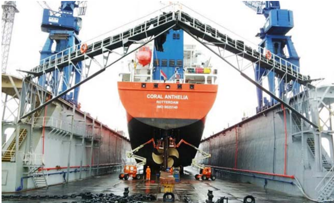
Dutch's Anthony Veder's Dwt 6,554 combined LNG/LPG Vessel " CORAL ANTHELIA " under rudder blade repairs in CernaVal Group Shipyards Algeciras Port. Photo : Enrique Pérez – CERNAVAL GROUP.
