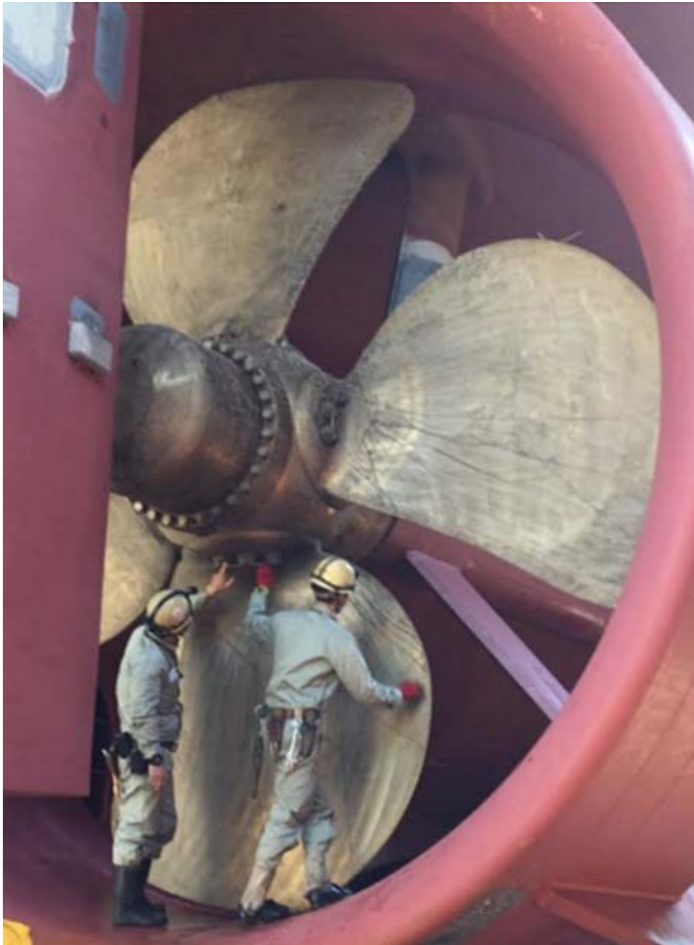
Inspection of the Starboard 5000 mm diameter propeller of the ALP STRIKER in drydock at Niigata Shipyard & Repair before polishing the propeller Photo : Leo Leusink ©
