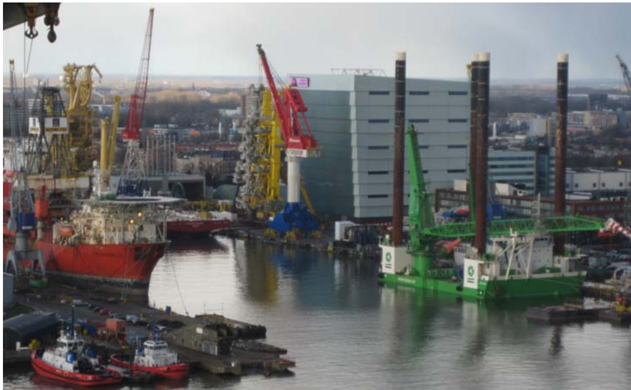
Huisman premises as seen from the EMAS vessel 'LEWEK CONSTELLATION'. In the foreground, the GEOSEA 'NEPTUNE' with a new upgraded boom. In the background, the 'CEONA AMAZON' with 570mt G-lay pipelay system. At the Huisman quay side the DOF/Technip 650mt Vertical Lay System. Photo : Rik van Wijngaarden ©
