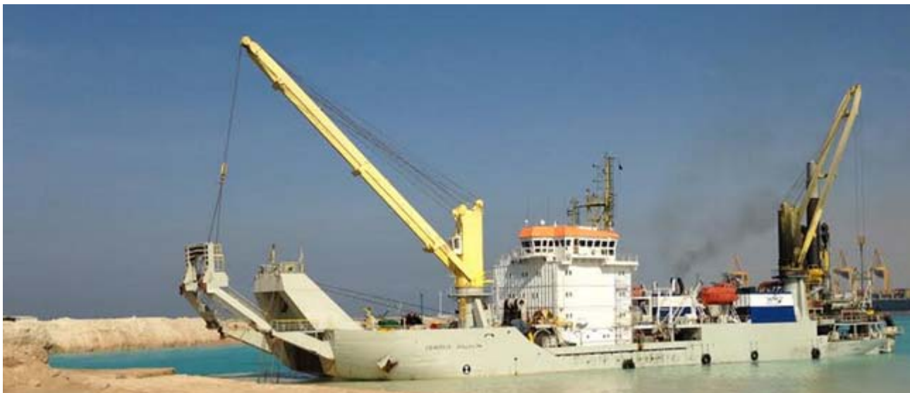
The former Boskalis CSD URSA , now named HUTA 14 seen operating in King Abdullah Port , Saudi Arabia
