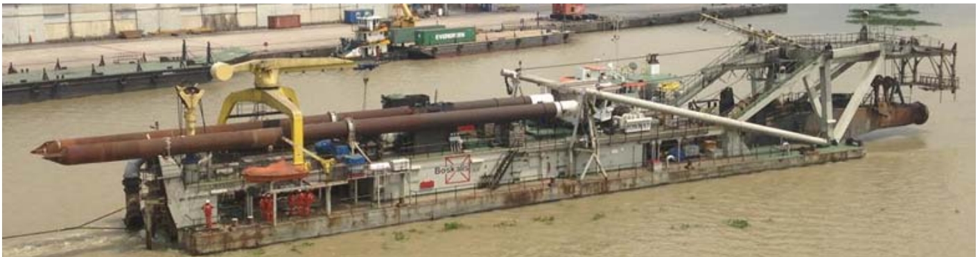
Boskalis' Cutter Suction Dredge JOKRA ready for transport to the next project on foreign shores.
