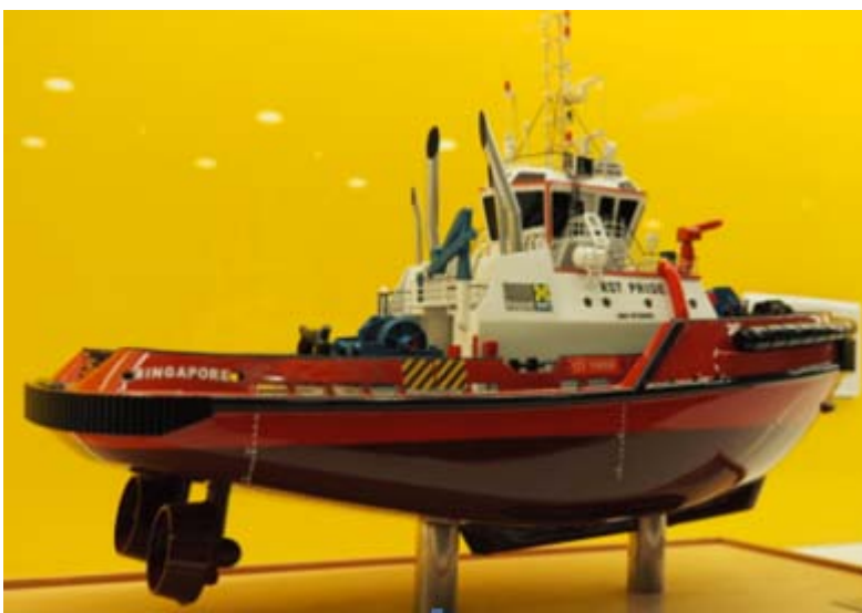
Ship-handling fenders at the bow consist of one row of 800 x 400 cylindrical fender at the main deck level, with 300 mm W fenders between the
