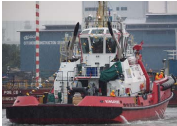
Ship-handling fenders at the bow consist of one row of 800 x 400 cylindrical fender at the main deck level, with 300 mm W fenders between the
