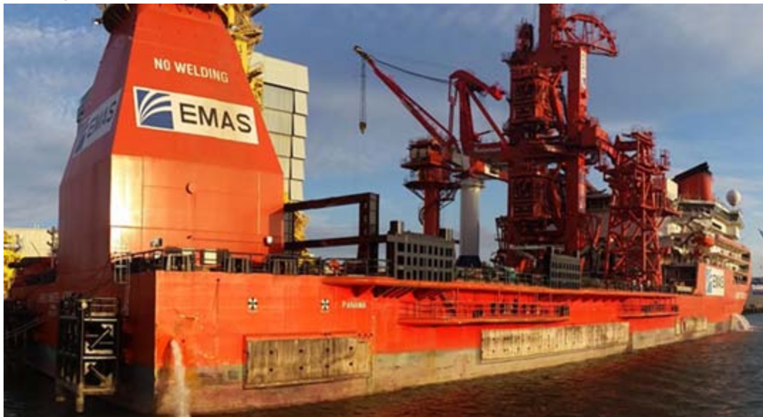
EMAS LEWEK CONTELLATION moored in Schiedam with the recently installed Huisman Multi Lay (for reel and flexlay) tower Photo : Floor van Kleeff ©
