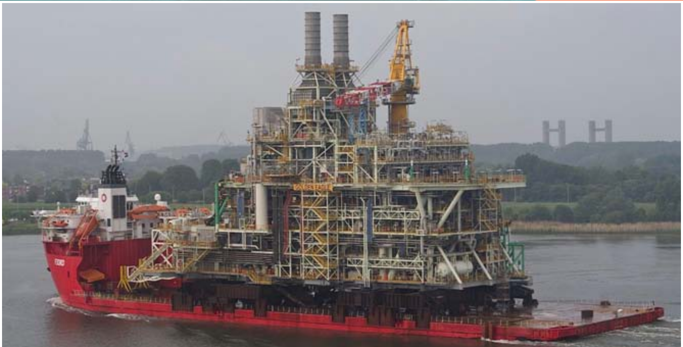
The FJORD loaded with the GOLDEN EAGLE topside passing Maassluis enroute to the Rotterdam Offshore Group in Rotterdam Waalhaven where some works will be executed . Photo : Monique Davis-Mulder (c)
