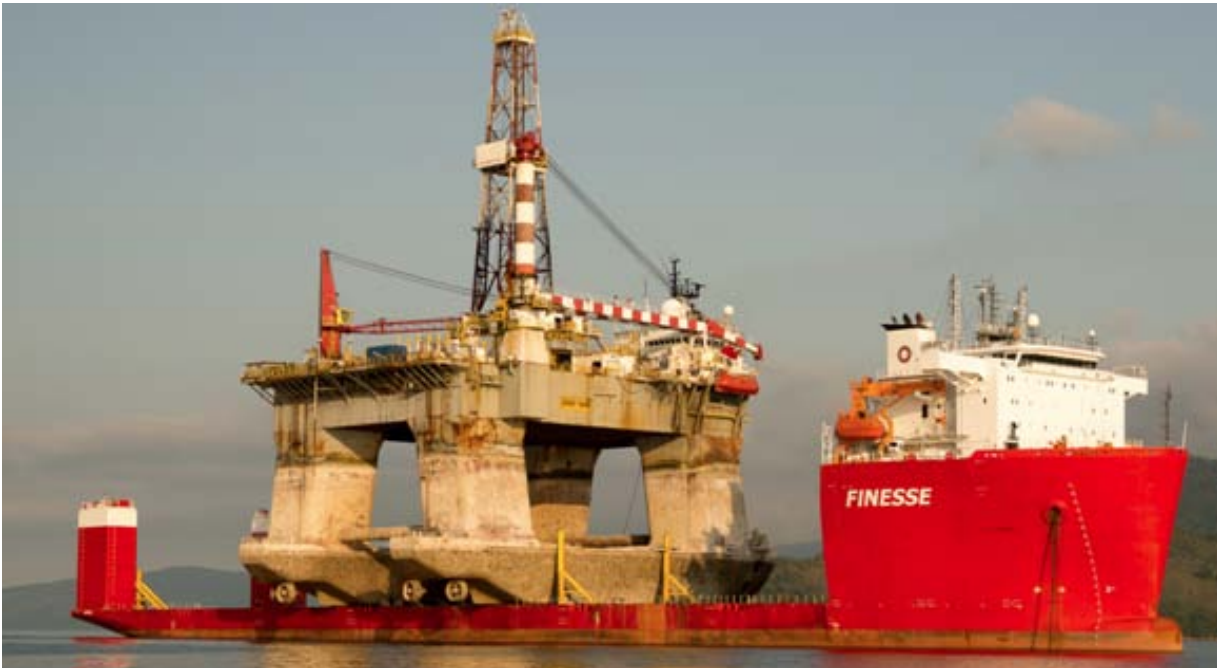
The FINESSE loaded the Semi submersible rig ENSCO 6000 in Angra dos Reis, Brazil Photo: Capt. Peter Kerkvliet - Master FINESSE (c)
