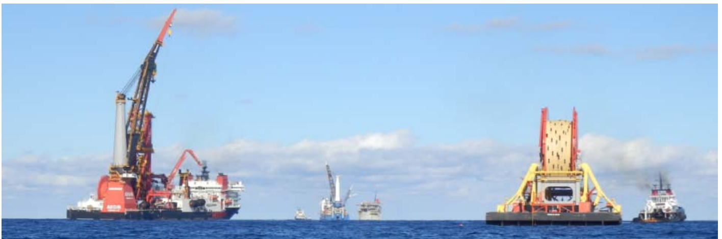
New reel arriving on barge towed by the Crowley tug OCEAN WAVE for DCV AEGIR . In the background the LUCIUS SPAR can be seen with the GLOBAL 1200 and supplier on her PS. – Photo : Edo Doeve (c)
