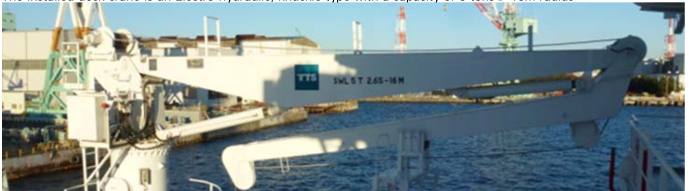
The installed deck crane is an Electro-hydraulic, knuckle type with a capacity of 5 tons@ 16m radius
