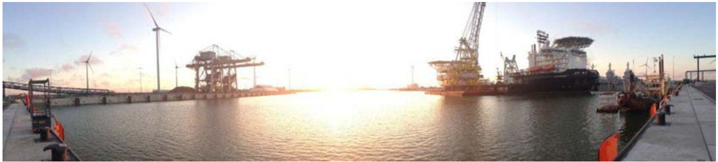
Barge with Borkum West Topside alongside Oleg Strashnov in Eemshaven.
