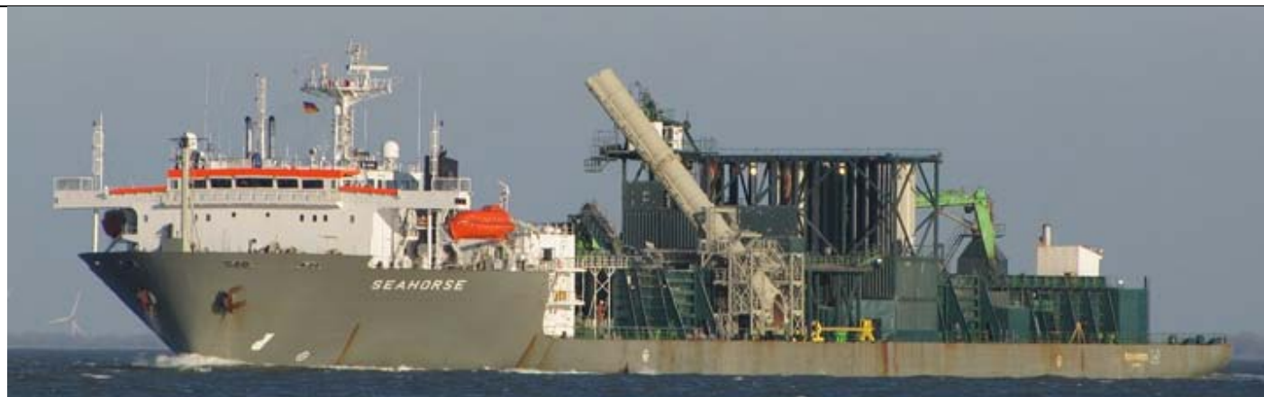
The stone / rock dumping vessel "SEAHORSE" departed from Cuxhaven heading to the Windfarm "Meerwind" in the North Sea - Photo : Maik Ebel ©
