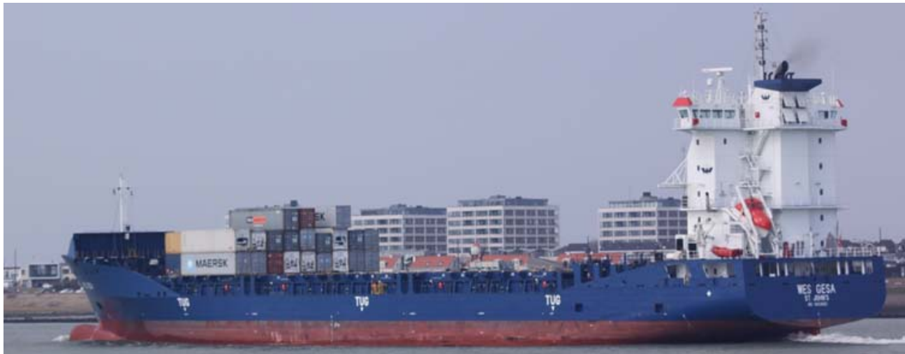
The 151 mtr WES GESA outbound from Rotterdam, the 13.200 DWT fully cellular container vessel is delivered 01—2012 by Jiangdong Shipyard in Wuhu under /hull No.: JD1000TEU-07 and is operated by Wessels reederei Photo : Paul Gerdes ©
