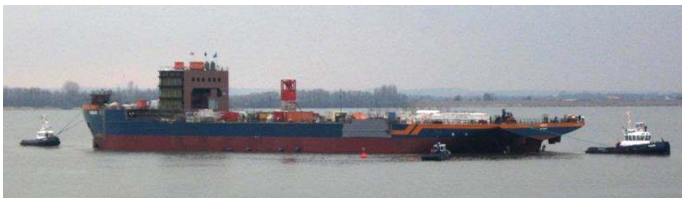
Spotted at the Elbe river near Hamburg the 139 mtr long new building offshore wind turbine transport and installation vessel AEOLUS under construction fitting out at Sietas Shipyard in Hamburg for Van Oord , the AEOLUS will be outfitted with a crane capable of lifting 900 tonnes. Photo : Boy Staats o/b Shoalway ©
