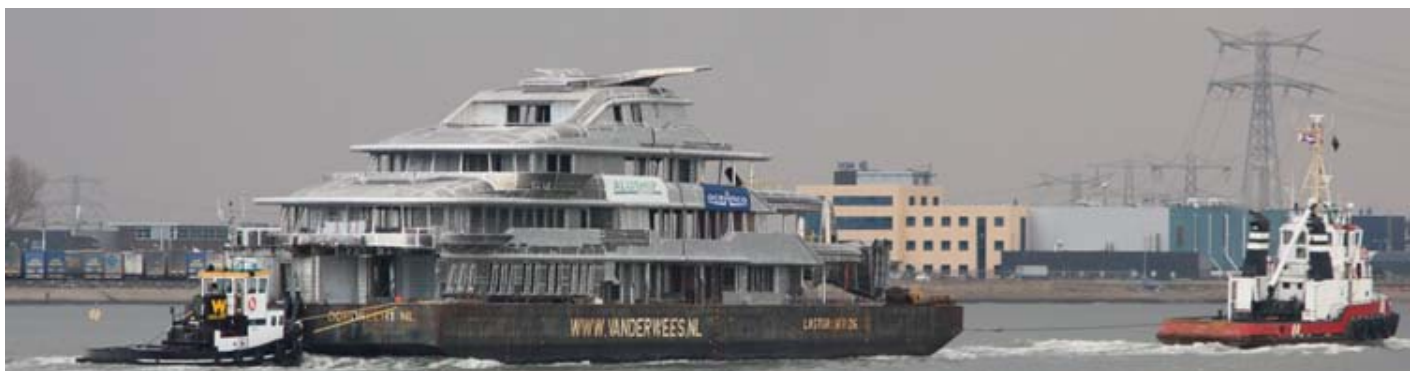
Wagenborg's WATERMAN arrived In Rotterdam with the Lastdrager 26 loaded with a large aluminium superstructure built by ALUSHIP for yacht builder OCEANCO
