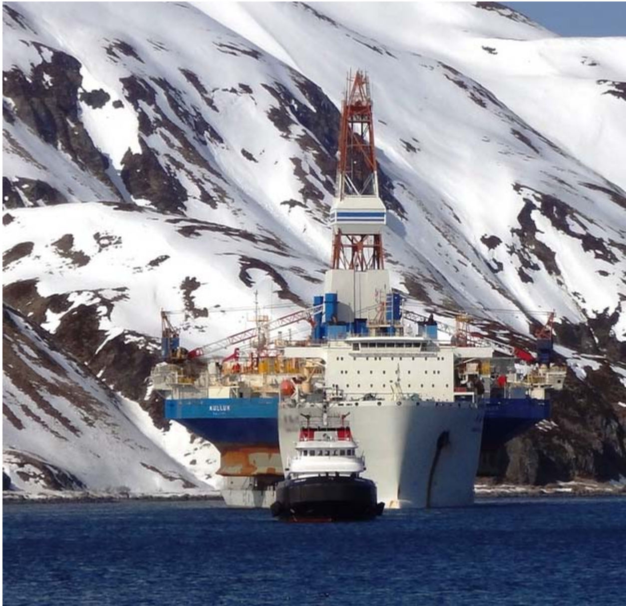
Crowley's tug OCEAN WAVE providing stand by and virtual anchor duties in manual and DP modes during the load-out and sea-fastening of the KULLUK on board the COSCO semi submersible vessel XIANG RUI KOU in Captains Bay, Alaska. Photo : Geoff Baker - Crowley Solutions based in Anchorage, Alaska.(c)
