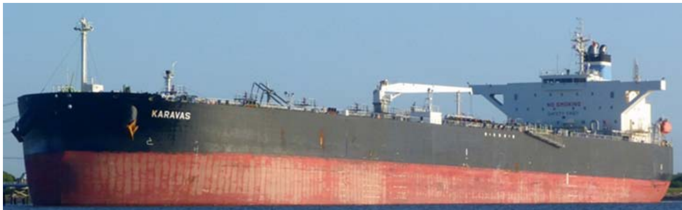
The 2010 built Crude Oil tanker KARAVAS moored in Brisbane, the 107.505 DWT 243.8 mtr long tanker is built at Tsuneishi Holdings Corp Tsuneishi Shipbuilding Co - Tadotsu shipyard under yard number 1422 – Photo : Chris Mackey - Southern Cross Maritime ©
