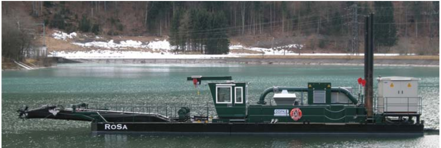
Even in Austria you can find a stationairy cutter dredger named " ROSA " working in the "Ausgleichbecken" Rodund in the province of Voralberg. Photo: Kees van Schie (c)
