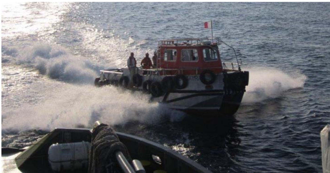
One CEMESA Cpy Service Boat acting as Pilot boat at YLNG terminal – Aluminium Catamaran build by Alnmaritec (UK)
