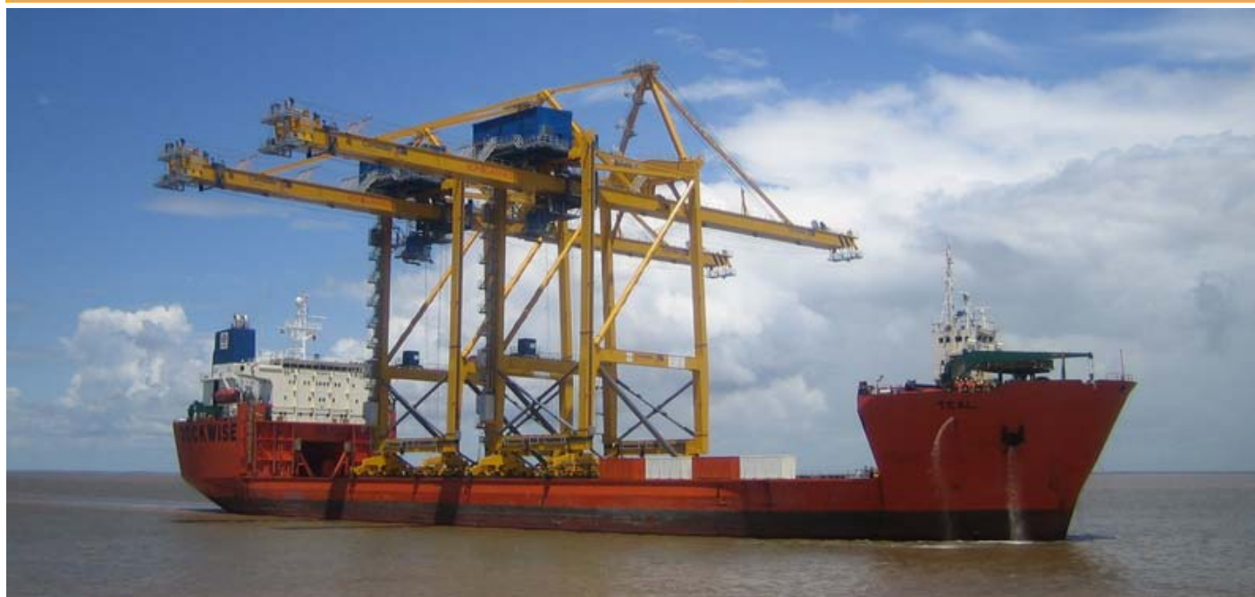
The TEAL of Dockwise seen on arrival at Beira, Mozambique loaded with two container cranes.
