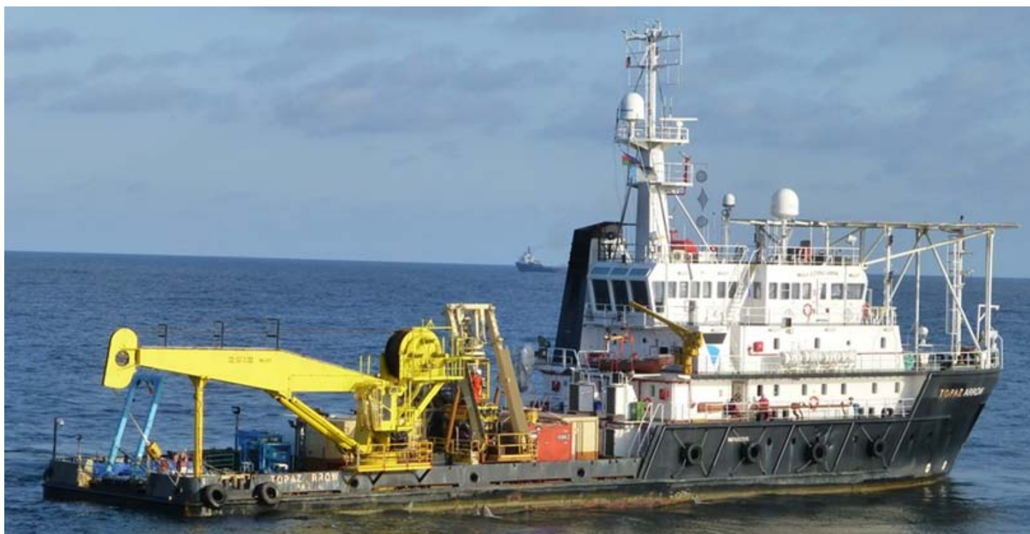
Azerbaijan, Caspian Sea , Chirag Oil Project , survey vessel TOPAZ ARROW in the process of TD monitoring the 16" pipe line for the PLB Israfil Huseynov Photo : Pieter C Holtes . BP/AIOC Marine Rep. ©
