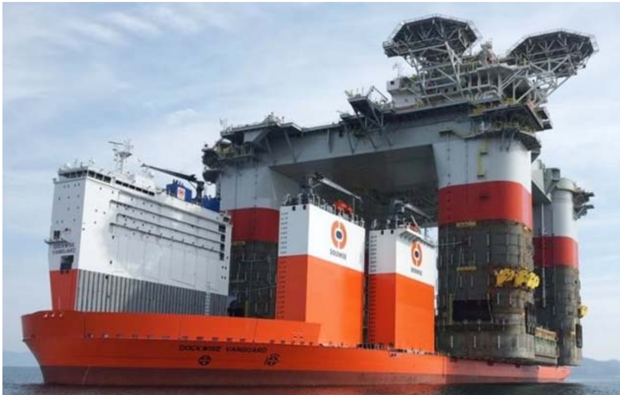
The DOCKWISE VANGUARD loaded at the Samsung yard in Okpo (Korea) her first cargo, the hull for the Jack/St. Malo semisub hub production facility for transportation to the US Gulf
