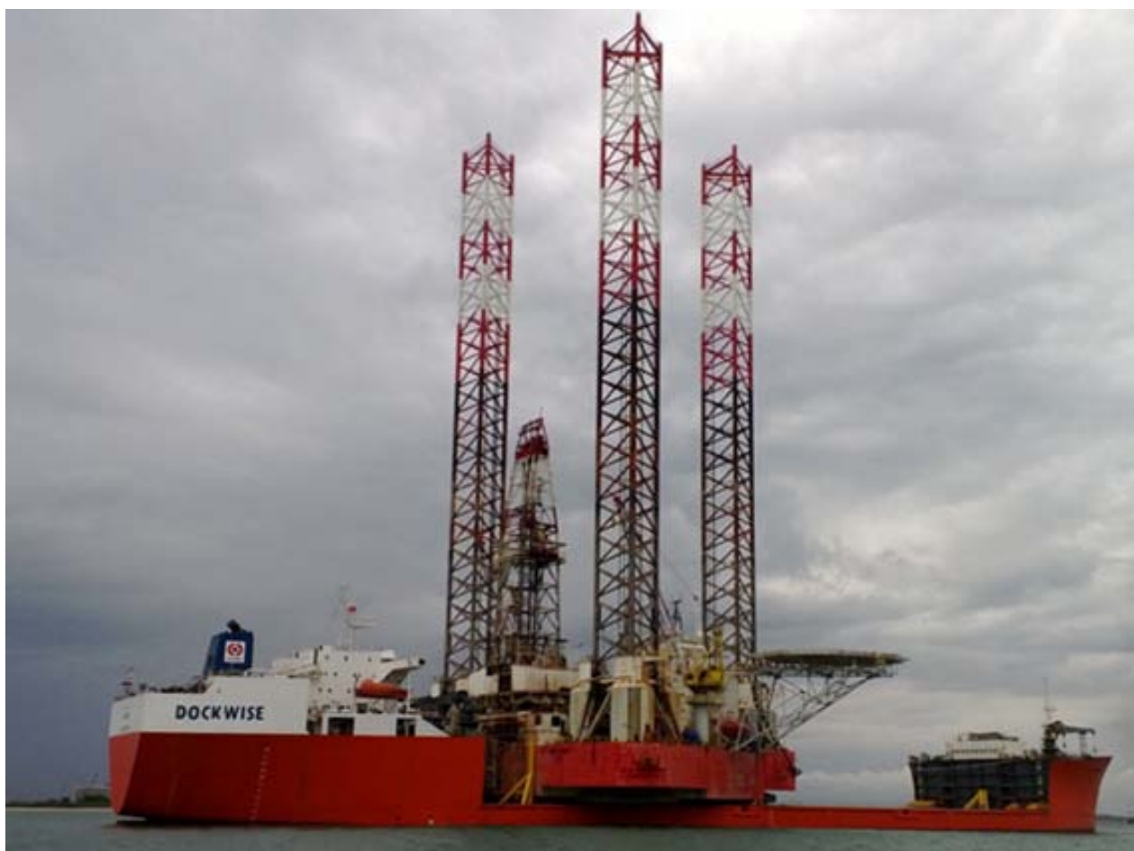
Dockwise TARGET loaded with the jack up WEST JANUS in Singapore- photo : Dockwise ©
