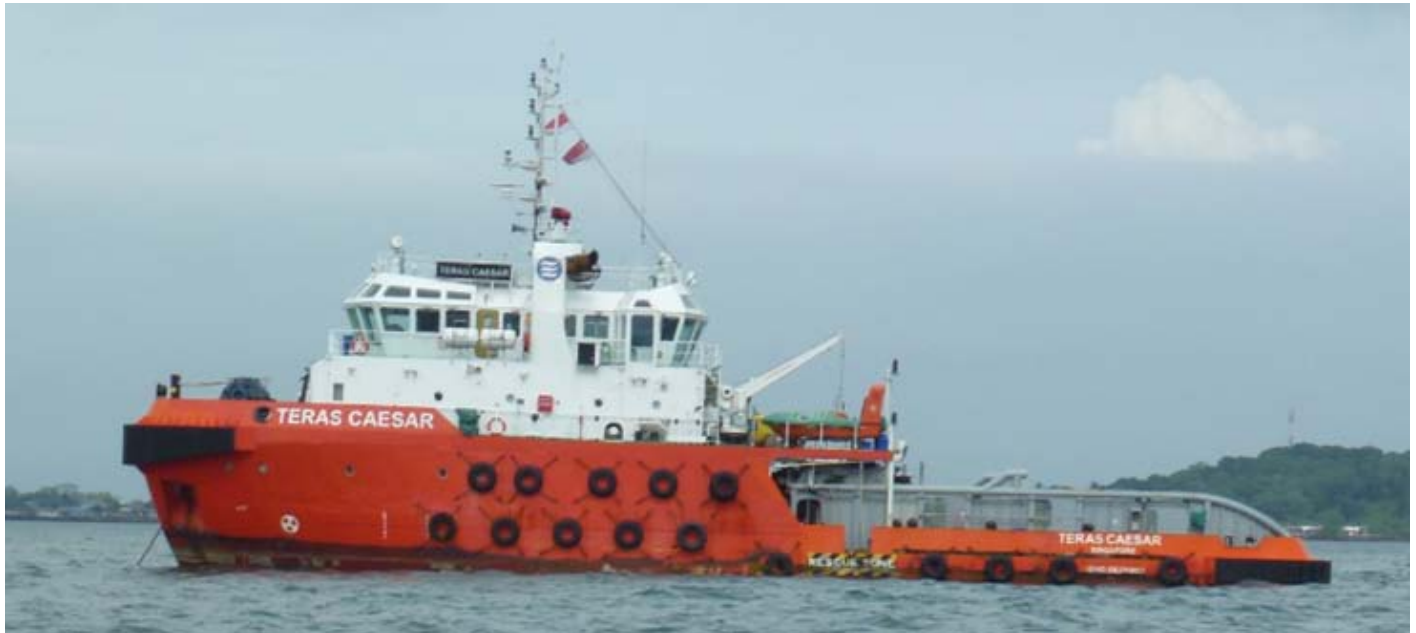
The 2012 CCCC BOMESC Marine Industry Co Ltd - Tianjin Yard built 45 mtr long TERAS CAESAR anchored off Batam – the Anchor handling tug is having a total installed power of 3,840kW (5,220hp)
