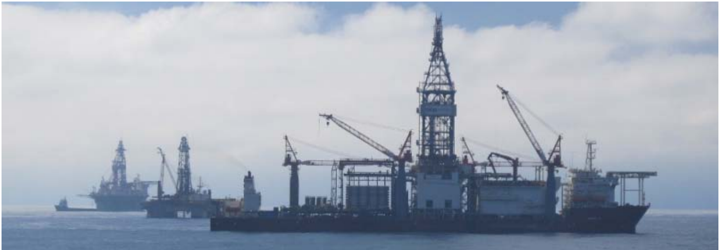
3 different types of MODUs seen from the rig Ensco 6004 . In the front: Odebrecht's drilling ship Norbe IX , in the middle: Semi-Submersible drilling rig Ensco 6003 and at the back: Sevan's cylindrical hull design drilling rig Sevan Brasil . Photo : Auke Ruijg - Campos Basin - Brazil. ©
