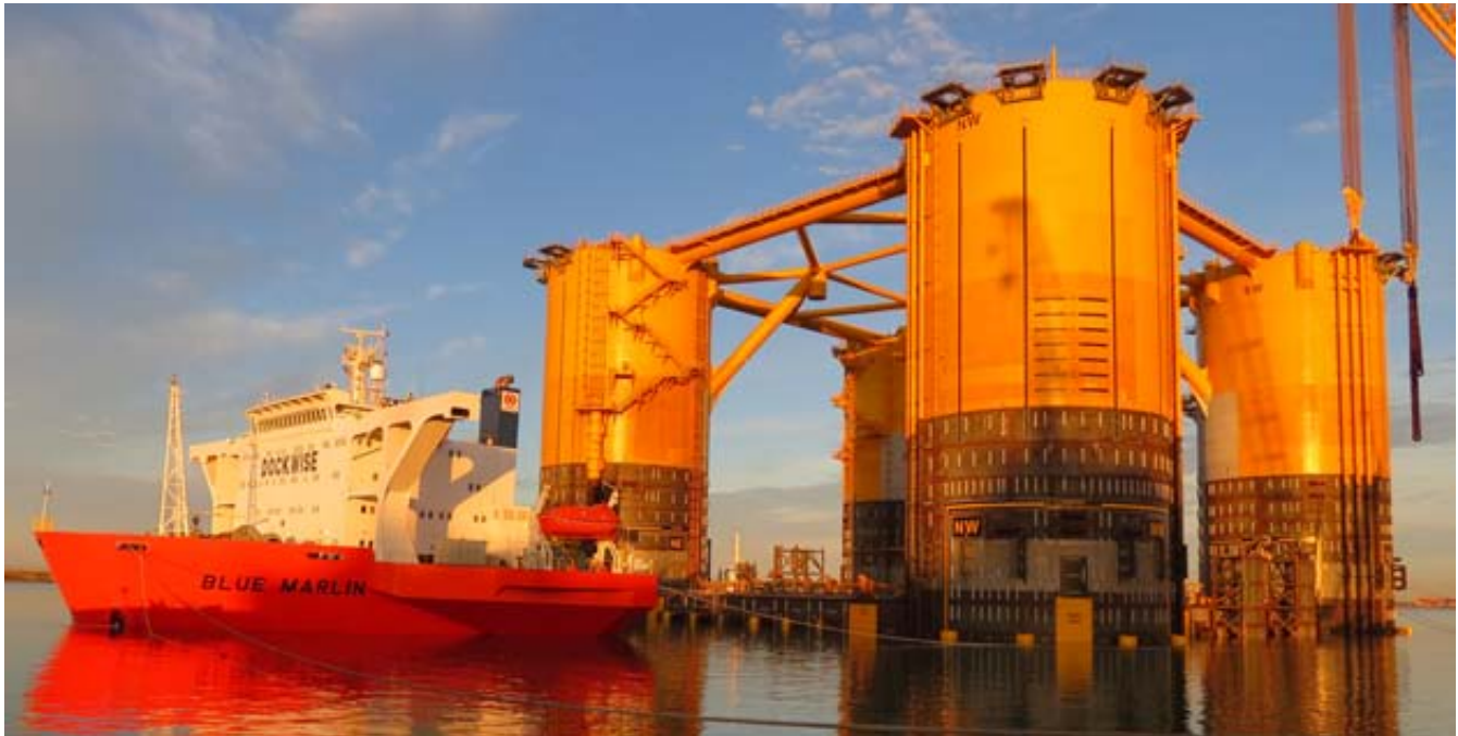
“BLUE MARLIN” at discharge draft, ready to offload the “MARS B OLYMPUS” TLP at Kiewit Offshore Services deep submergence area Ingleside, Texas. Photo : Tracy Horton – Operations Manager ProBulk LLC, as agents for Dockwise Shipping BV ©
