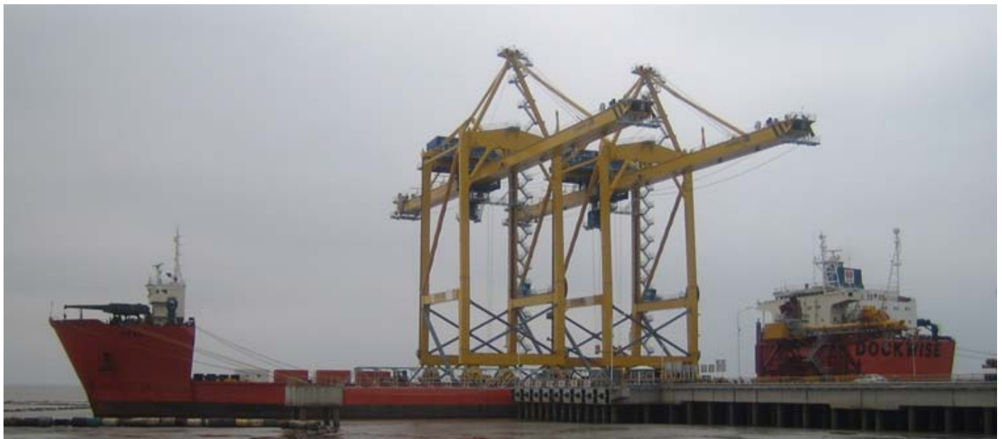
The TEAL of Dockwise at Haimen, China. Loaded with two container cranes -Photo : Andre Korver ©
