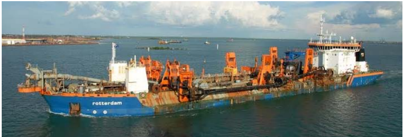
Van Oord's TSHD ROTTERDAM operating in Darwin at the Ichthys project as seen from the TSHD QUEEN OF NETHERLANDS Photo : Danny Plug (c)
