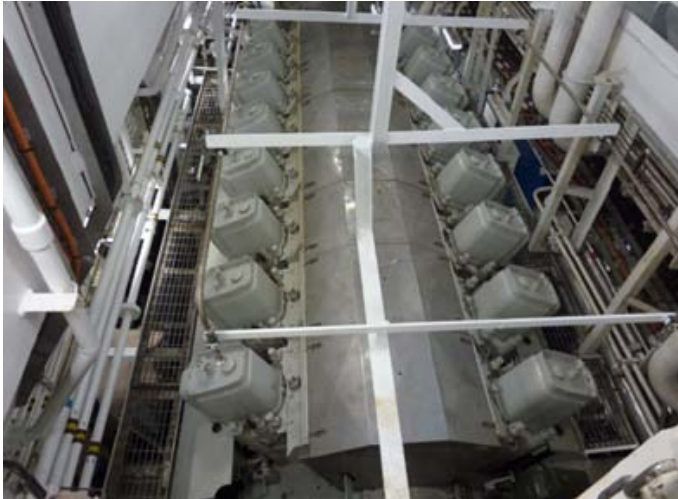
Left and below seen one of the 2 enormous MAK 16 Cy. 10,877 hp main engines
