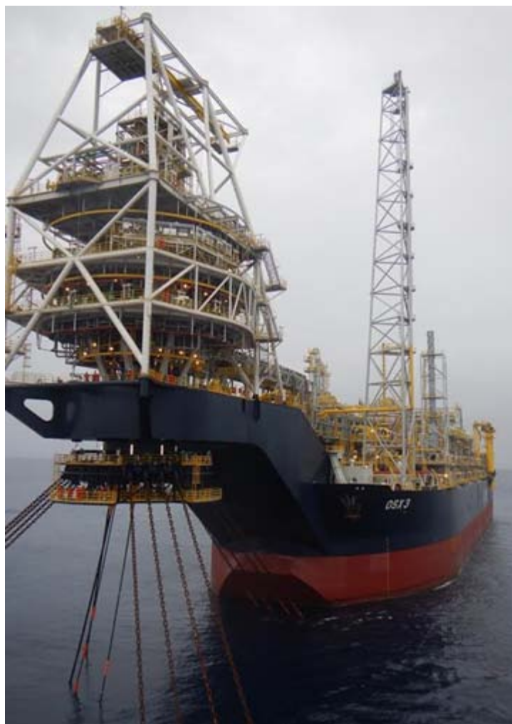
The transfer of raisers layed by AKER WAYFARER on the seabed to the FPSO OSX 3 at the Tubarao Martelo Oil Field in Brazil. Photos : Sondre Butler Gangdal ©
