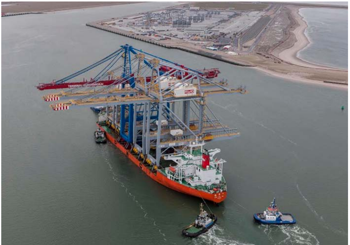
The ZHEN HUA 25 entering Rotterdam Maasvlakte II loaded with the new Container cranes for the Rotterdam World Gateway
