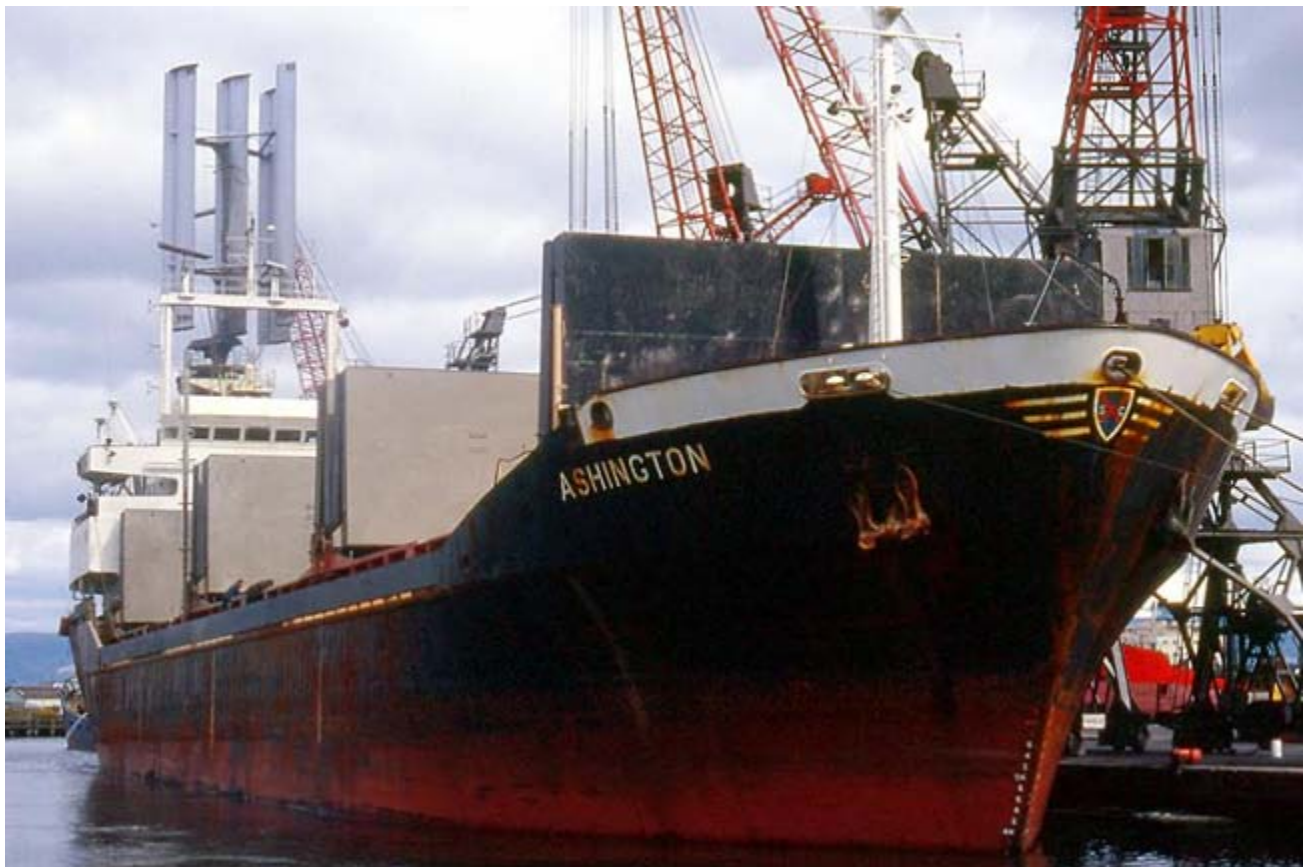
" ASHINGTON " berthed East Wall, Grange Dock, Grangemouth on 17/5/1988 , she is discharging a cargo of coal for Longannit Power Station. The ship was fitted with experimental sails above the accommodation. Photo : Iain Forsyth ©
