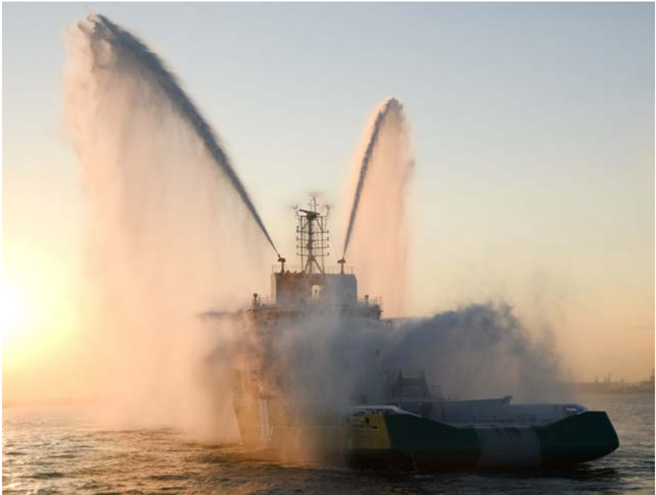
The TERASEA EAGLE testing her Fi-Fi equipment in Tokyo Bay – Photo : POSH Terasea (c) CLICK on the photo to see the High resolution version
