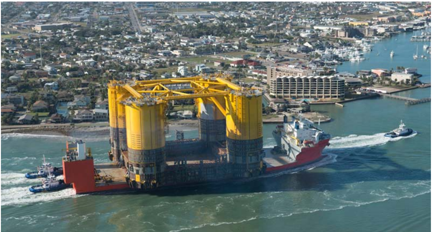
DOCKWISE "BLUE MARLIN" (76,292 SDWT) arriving from SOUTH KOREA inbound passing ARANSAS PASS, CORPUS CHRISTI WITH THE SHELL MARS B OLYMPUS HULL (32,541 M/TONS) – photo : BOB REDDING, REDDING COMMUNICATIONS. ©
