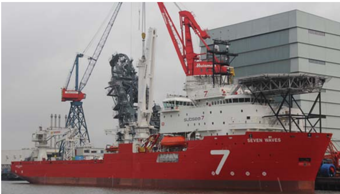
At the Huisman premises in Schiedam the 400 tons crane was installed onboard the SEVEN WAVES
