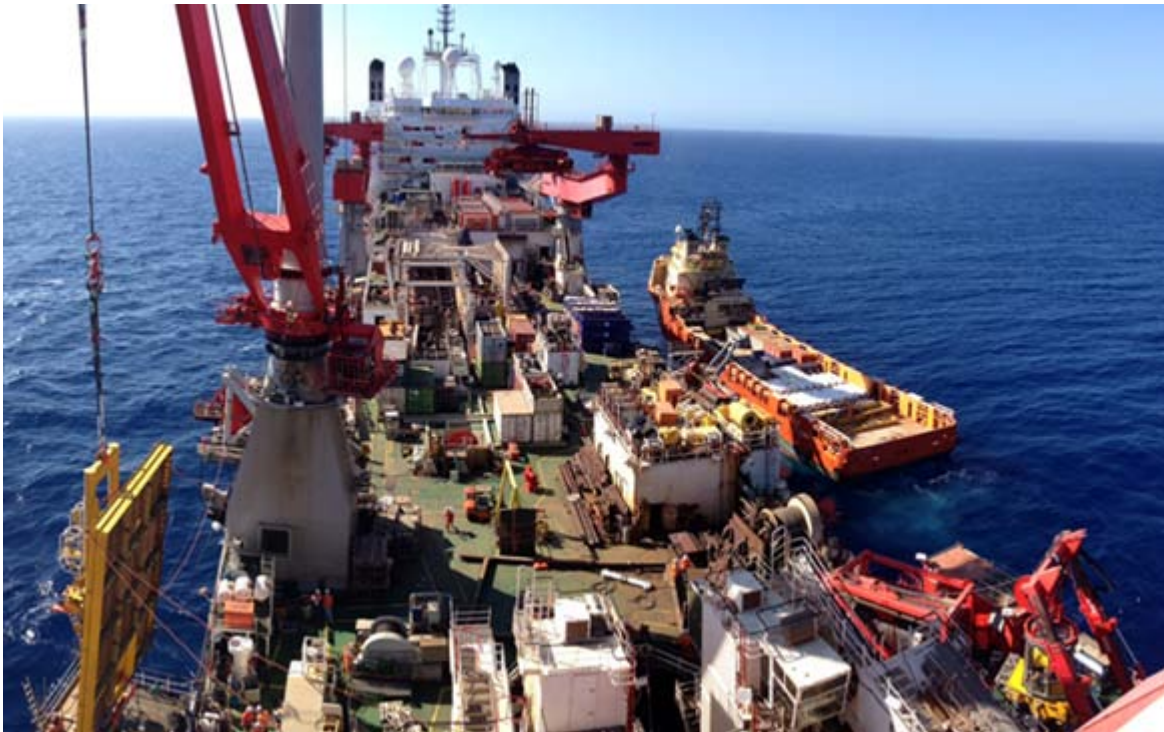
PSV Toisa Solitaire alongside PLV Solitaire during PLET-installation on the Jansz project, Western Australia, offshore near Barrow Island. Photo : Erwin de Vries ©
