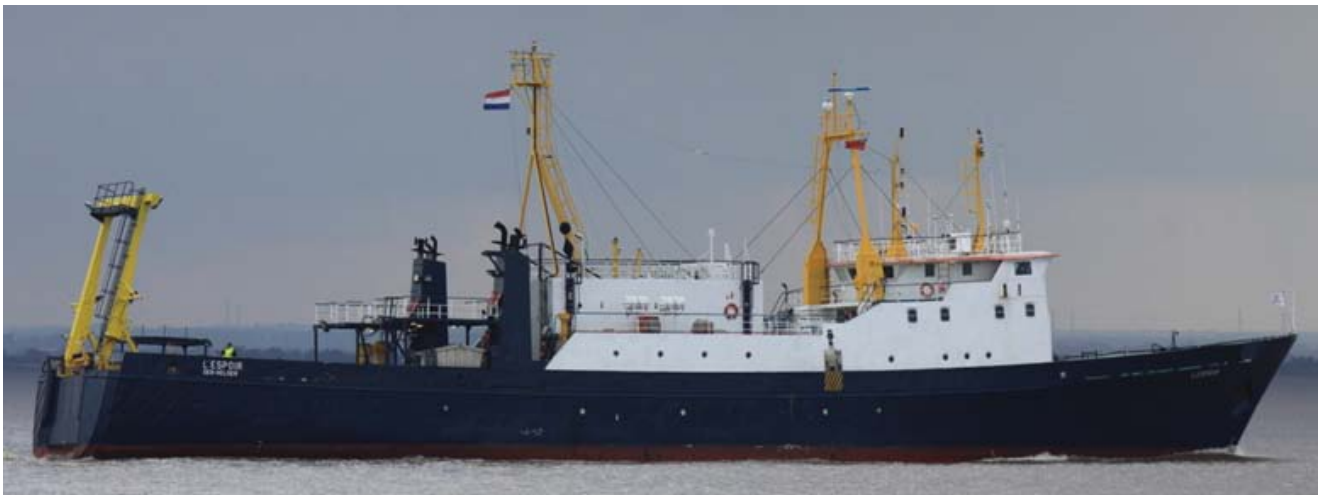
The 1971-built research vessel L'ESPOIR arriving at Hull from Lowestoft. Registered in Den Helder she is operated by Tranship BV . She was built at Messina by Cantieri Cassaro as a stern trawler but converted to a seismographic research vessel in 1977. Photo : Simon Smith ©
