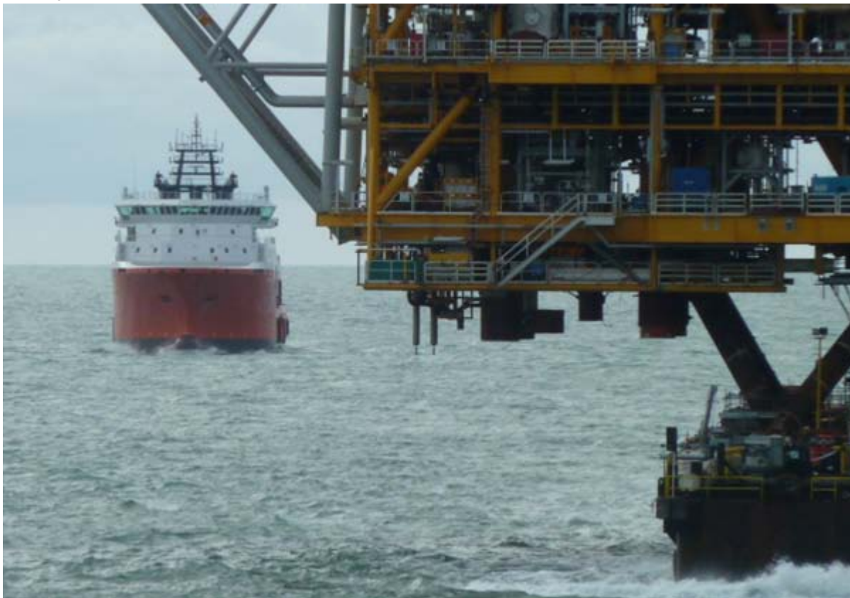
The SAIPEM 45 loaded with the Zawtika Topsides enroute from Sembawang to the M-9 field in Myanmar, with the " PACIFIC DOLPHIN " escorting the transport in the Malacca Straits Photo : Capt. Hans Bosch ©
