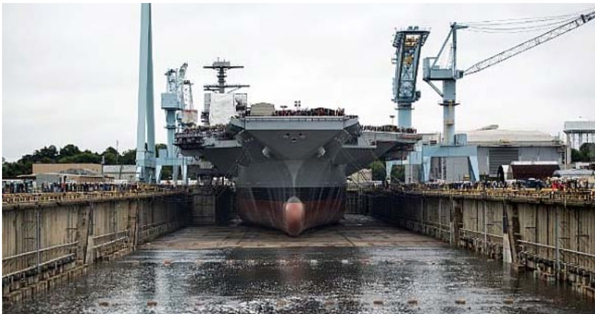
Newport News Shipbuilding begins flooding Dry Dock 12 to float the first in class aircraft carrier, Pre-Commissioning Unit GERALD R. FORD (CVN 78) . Photo : US Navy
