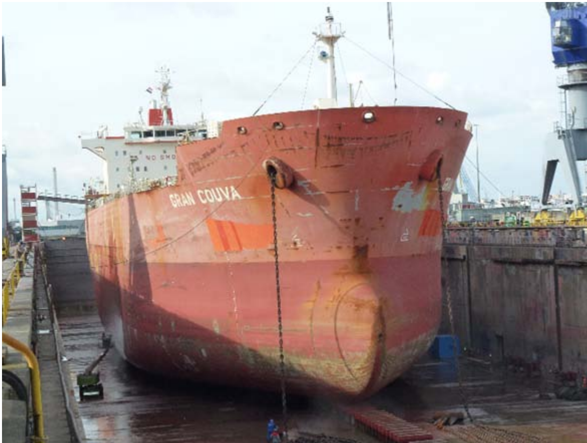
Mt " GRAN COUVA " (Dim: 183,21 x 32,26 x 12,20 mtr. ) at Damen Shiprepair Rotterdam drydock number 7 for outside hull cleaning and painting .Photo : Joop Bartels ©
