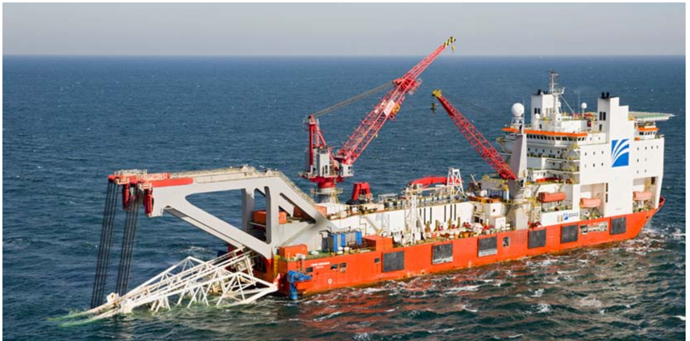
EMAS pipelaying vessel LEWEK CENTURION during the installation of a pipeline towards the Q13-A platform offshore Scheveningen (The Netherlands)
