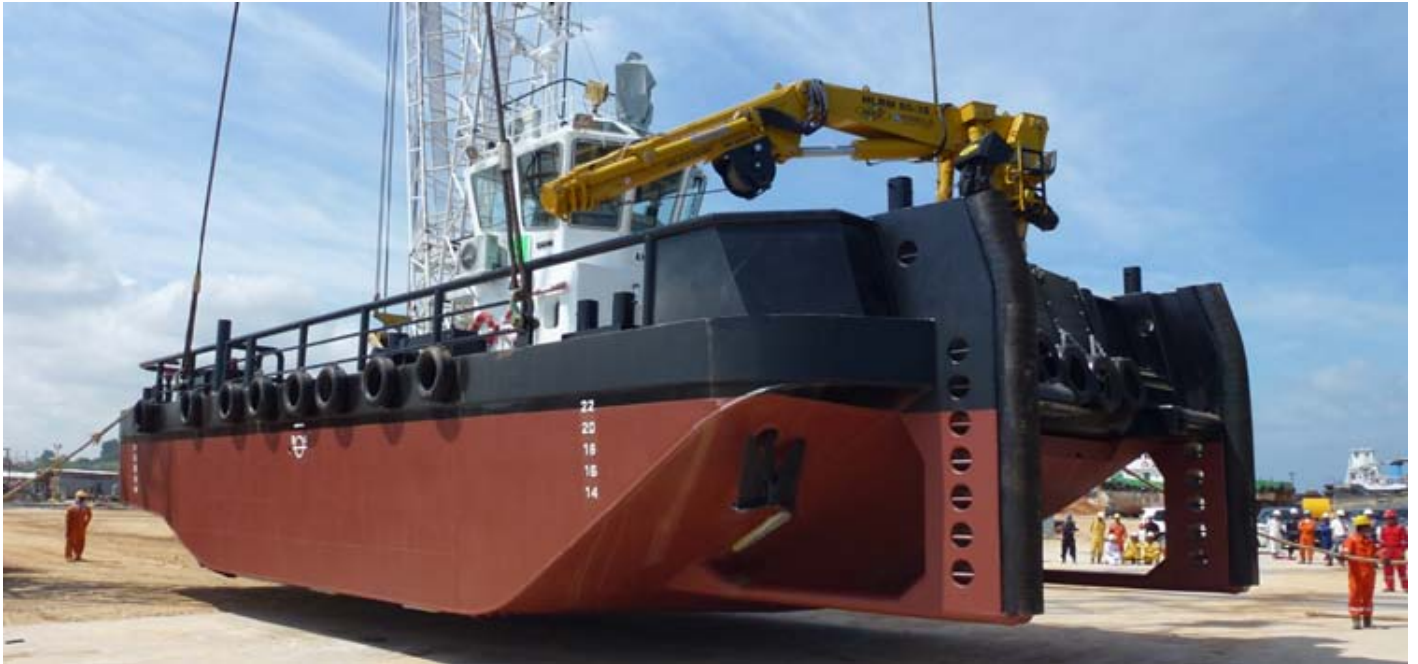
The 18.9 mtr long and 8 mtr with ANGIE is powered by 2 Caterpillar engines of 600 BHP each
