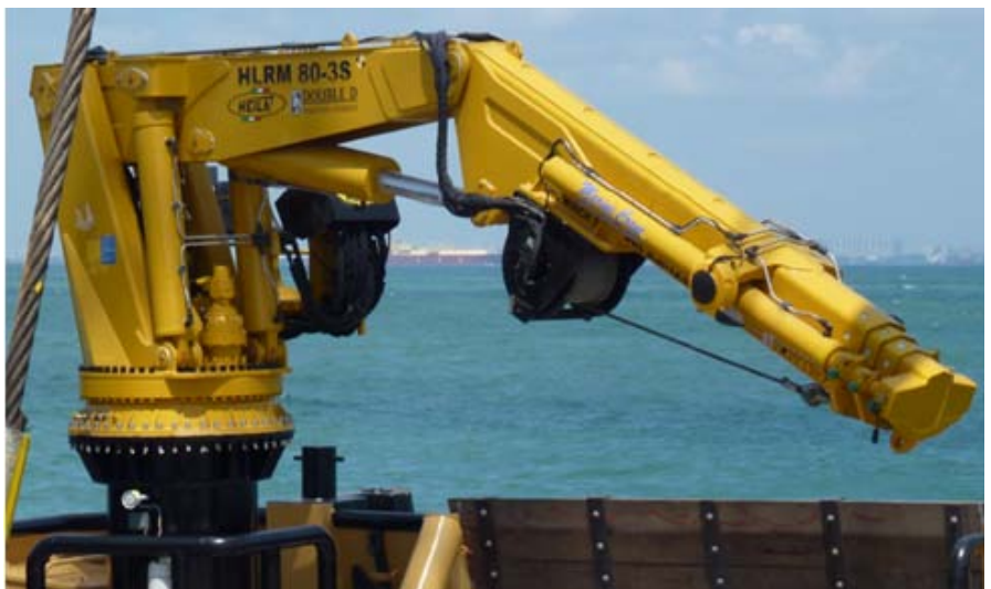
at the bow a HEILA HLM 80-35 hydraulic crane with a capacity of 6,4 ton at 10-18 mtr is installed.
