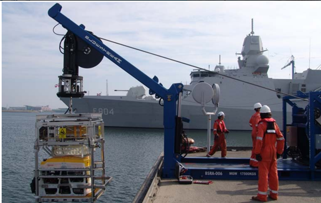
Bluestream Offshore testing a brand-new Seaeye Cougar ROV and TMS at the Den Helder Naval Base – Photo: Paul Schaap ©
