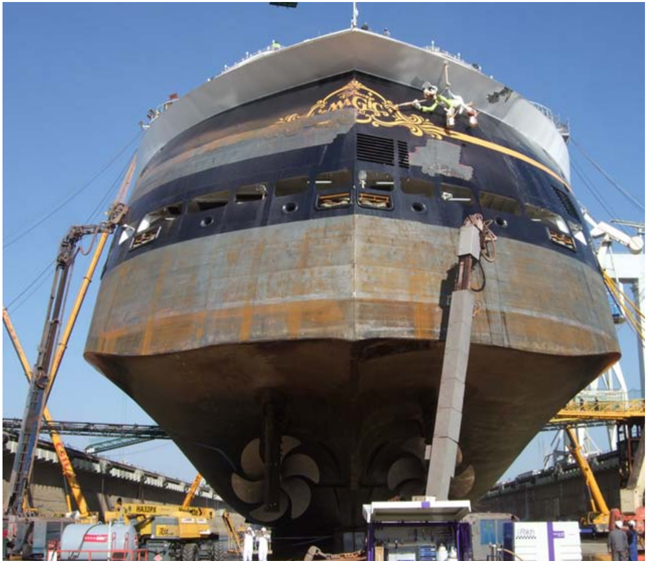
The DISNEY MAGIC in drydock in Cadiz (Spain) where the Outside hull and topsides are getting Hydrojetted and the Yard will apply 4 new layers paint on the ship in 4 weeks.
