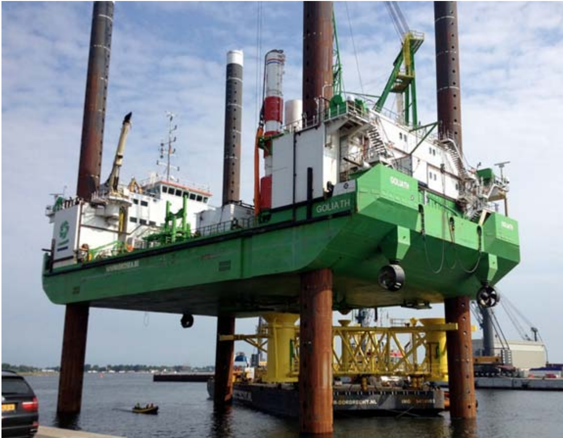
The jack-up GOLIATH in Rostock whilst the tug SEA ALFA is pushing the barge underneath the jack up during the installation of the special Piling Frame Photo : Wim Holland ©
