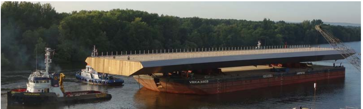
The tug DUTCH POWER connecting to the SARENS BARGE VEKA 3303 , heading for Sundsvall (Sweden). The barge loaded with a 132 mtr bridge section, is just pulled out with winches, assisted by FAIRPLAY 4 (at the front) + FAIRPLAY 7 (on the aft) from the loading area in Stettin (Poland) – Photo : Ion Theuerkauf ©
