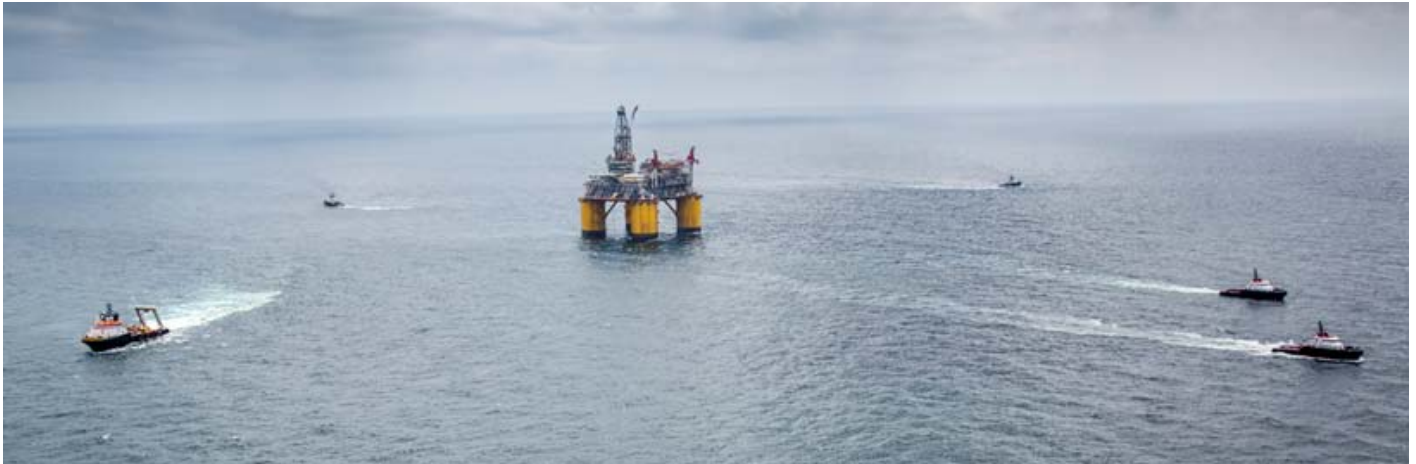
Crowley Ocean class tugs OCEAN WAVE, OCEAN WIND, OCEAN SUN with Boskalis UNION MANTA contracted direct by installation contractor made up in the station keeping Star Pattern. OCEAN SKY performing duties as standby tug. Photo : Tim Burdick ©
