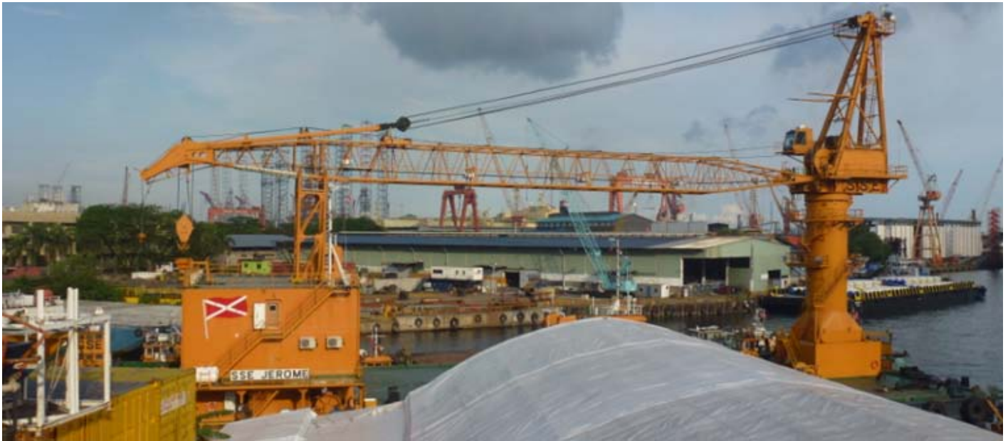
The latest fleet addition to SSE is the 2013 delivered crane barge SSE JEROME . equipped with an 150 ton SWL @ 23 mtr outreach crane , click here for the complete fleet list off SSE Photo's : Piet Sinke ©
