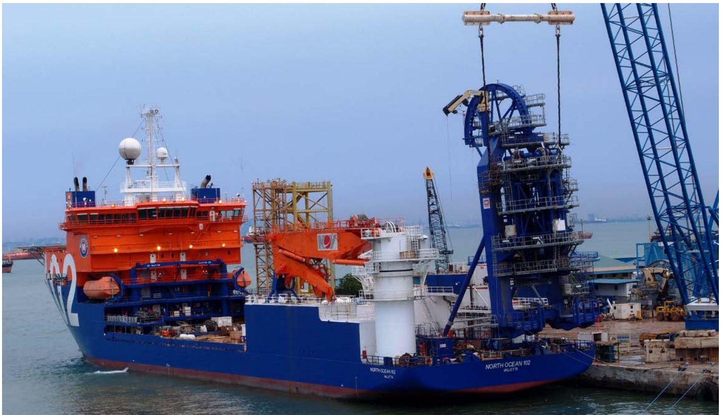
The LAY VESSEL NORTH OCEAN 102 having her new IHC Merwede Flexi-lay tower installed at the BMB in Batam, Indonesia – Photo : Capt. Jelle de Vries ©
