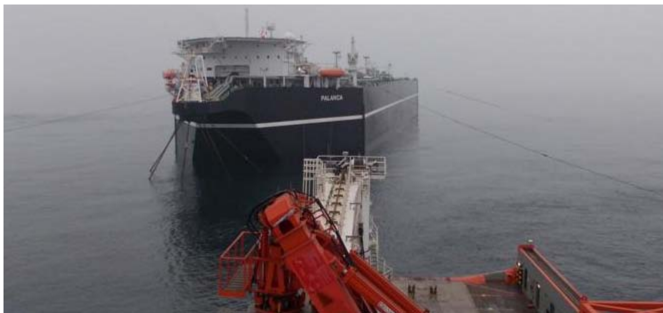
MPSV LEWEK FALCON ( EMAS AMC, Singapore) – installed FSO PALANCA ,anchored by 6 mooring chains in 44 m water depth ob Block 03 Offshore Angola. Photo : Vitaliy Nosychenko - MPSV Lewek Falcon ©
