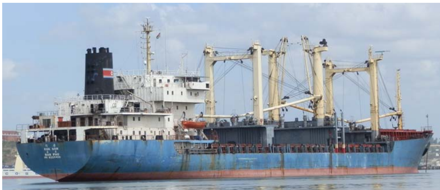
the mv KUK SAN at the inner anchorage at Mombasa, A North Korean general cargo ship built in the former DDR in 1982, IMO# 8225436. The derricks could now be a nightmare, not often seen these days, 125 tonne heavy lift removed. Photo : DAVID FIDDLER - Consultmarine SA cc ©
