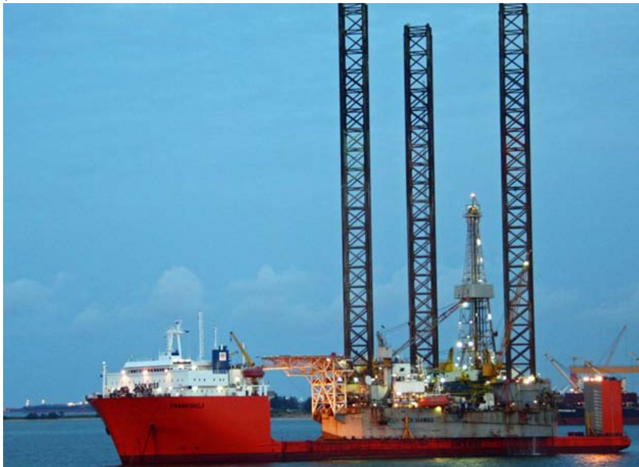
Dockwise TRANSSHELF during the seafastening of the KEY HAWAII prior departure from Singapore West Jurong anchorage Photo : Capt. Neil Johnston – Master Salviscourt ©
