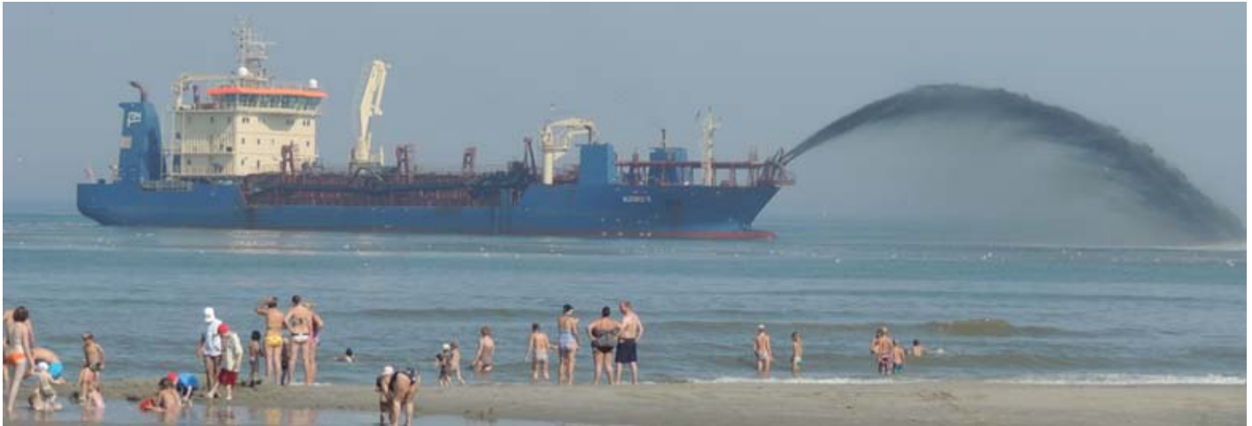
The Danish flagged TSHD NJORD R rainbowing at the discharge location near the Dutch town "s Gravenzande.
