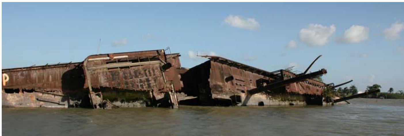
The wreck of the GOSLAR in the Surinam river near Paramaribo, the vessel was scuttled by the Germans in 1940 during a salvage attempt the vessel broke her back as can be seen at the photo : Photo : Hans ten Katen Sr. ©
