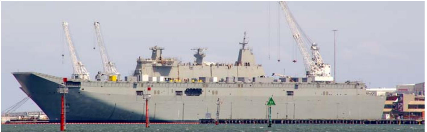
CANBERRA under construction at Williamstown Dock Yard at Williamstown Melbourne. All works above deck level has been constructed in Australia Photo : Bill Barber ©
