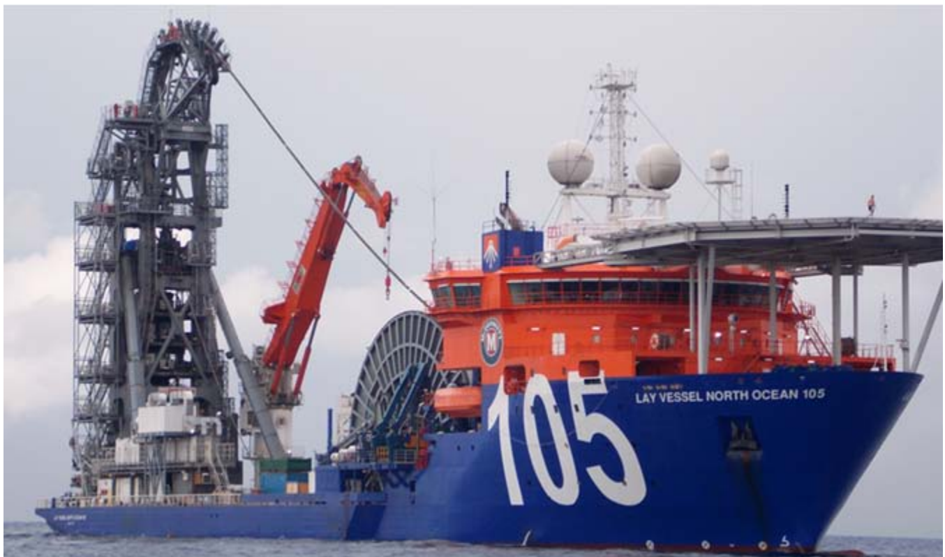
The McDermott Lay Vessel North Ocean 105 testing the rigid reelpipe laysystem off East Malaysia in 1000+ mtrs - Photo : Capt. Jelle de Vries ©
