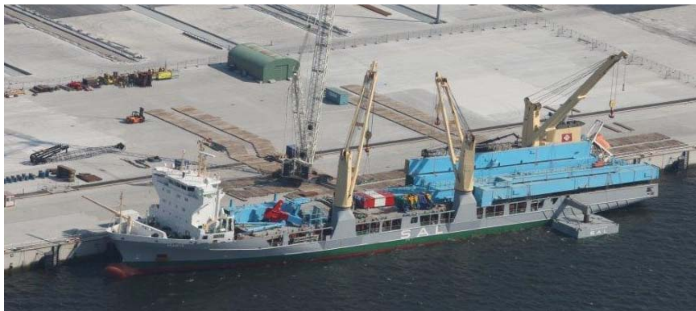
SAL's MARIA moored in Rotterdam at the APMT terminal at the new Maasvlakte II loaded with new Cargotec Ship to shore cranes, this cranes are built in China and assembled at the Maasvlakte
