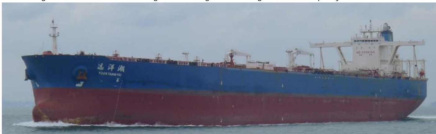
The 2010 built 297.305 DWT Crude Oil tanker YUAN YANG HU passing the Singapore Straits, the 330 mtr long and 60 mtr width tanker is built at Dalian Shipbuilding Industry Co Ltd - Dalian LN (No 2 Yard) under hull No.: T3000-22 and is owned by COSCO and powered by 1 MAN-B&W - Dalian Marine Diesel Co Ltd China built 7 cylinder 34,643 hp engine for a Service Speed of 15.8kts – Photo : Paul Firet ©
