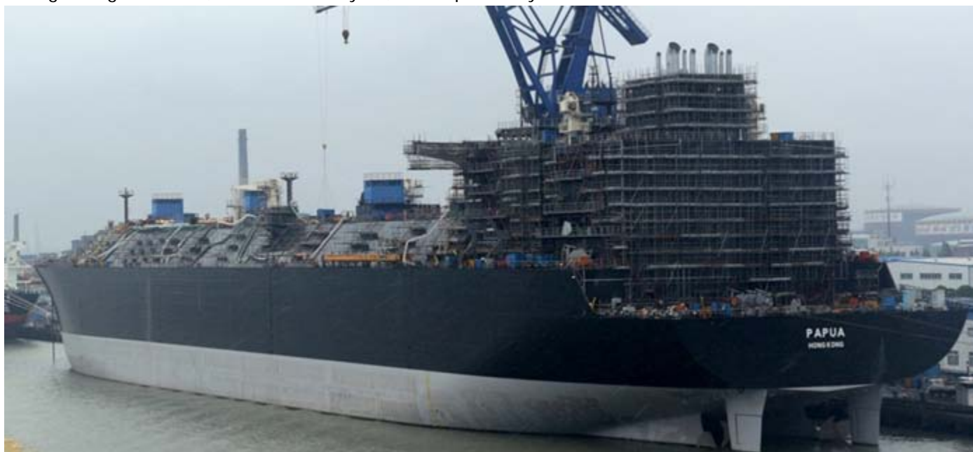
The LNG tanker PAPUA under construction at Hudong-Zhonghua (China)
